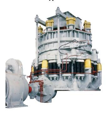
Based on the study conducted on the need in crushing machinery a number of basic modifications has been developed to process materials with lumps up to 1200 mm and output of  $150 \text{ to } 2000 \text{ m}^3/\text{hr}$ .
