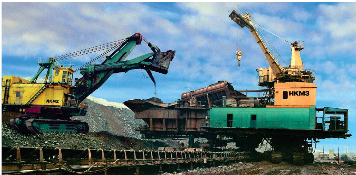
ДПА-2000 Self Propelled Crushing-and-Reloading Unit
