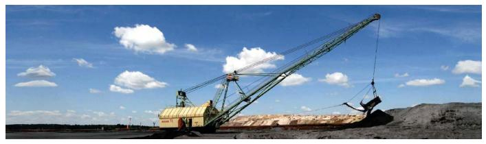
Walking draglines feature the full-revolving electric-operated earth-moving walking machines fitted with dragline working equipment.
