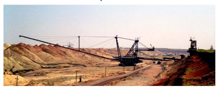
Spreader is a mining-and-handling machine capable of moving in a walking mode, on rails or on tracks, designed to haul the overburden to the dumps.
