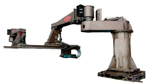
Taphole opening machines are designed to open the blast furnace tapholes at heat tapping. They are installed in the blast furnace casthouse.
