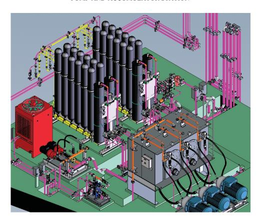
Pump-and-accumulator station is designed for servicing of taphole plugging/opening machines and laundercover lifting manipulators. It consists of hydraulic tanks, pumps unit, hydraulics columns, air (nitrogen) preparation plant, compressor.
