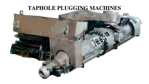
Iron taphole plugging machines are designed to plug the blast furnace tapholes with the refractory filler material. They are installed in the blast furnace cast house.
